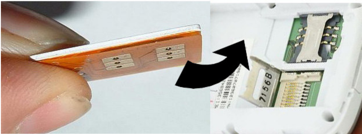
Step ,Insert both of the SIM and SIM dialer into your mobile phone SIM holder slot together.(Keep justification for both SIM and Dialer)
