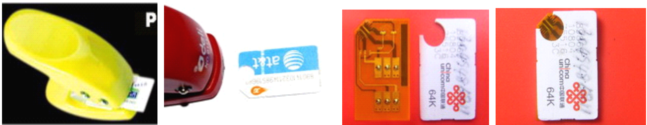
1,Punch the SIM a hole same location to the IC on V400 together
